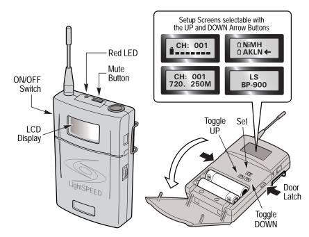
• Turn the transmitter ON by pressing and holding the Power button on the side *(approximately 2 seconds)*. The LCD display will appear.
